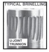
**False Brinelling:** Considered not to be a case of brinelling at all. Needle rollers sometimes polish the trunnion or needle cups so that they appear to have brinelling. Even during low kilometeres. To determine false brinelling, rub your thumbnail across the surfaces. If you do not feel any roughness or indentations, then the condition is false brinelling. False brinelling does no damage to the metal surfaces and the part is still okay for continued service.
